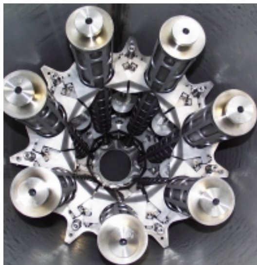
Figure 3 - Canister inside view showing rack, cans and magazines before pouring glass
