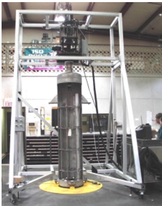
Figure 6 - Canister Loading Robot Mockup
