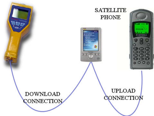
Figure 2 - Schematic of Shipboard Portion (Phase 1)
