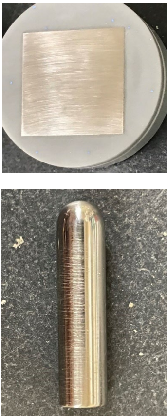
Figure 2-5: Examples of A537 square (top) and bullet (bottom) electrodes used for CPP experiments.
