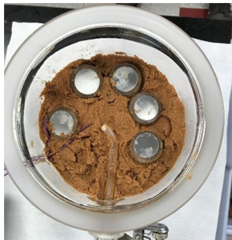
Figure 3: Image of the mass-loss coupons placed inside migration experimental unit
