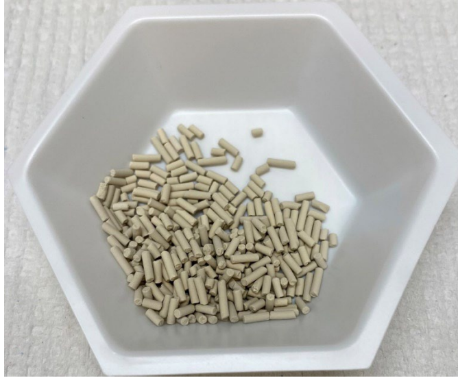
Figure A-7. Granular Zeolite 10A (13X)
