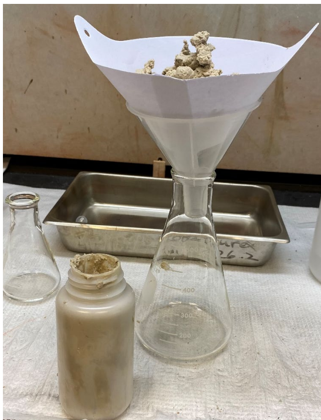
Figure 2-2. Paint filter/setting test setup with Aquaset II.
