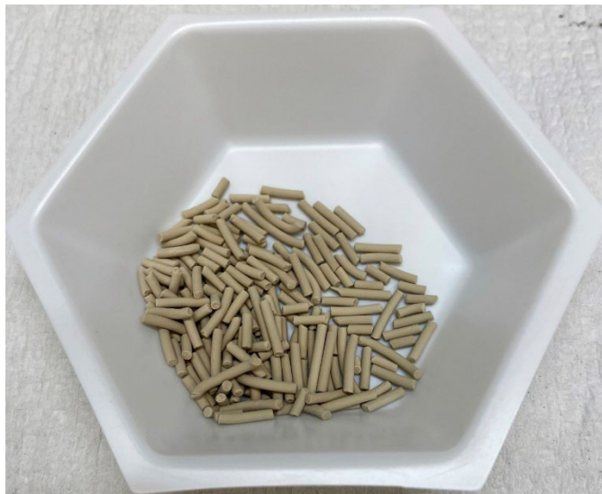
Figure A-6. Pellet Zeolite 4A
