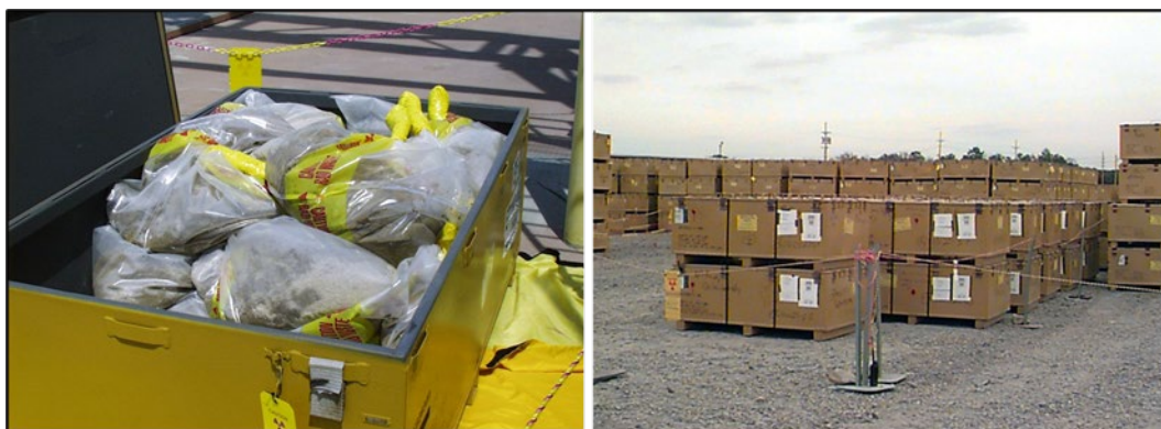
Figure 4-57. GT-73 Spent Resin in a B-12 Box from the ETF (left) and Spent Resins from the F-Area and H-Area Groundwater Treatment Units (right)
