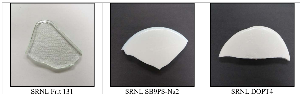
Figure 4-1. Images of as-poured glasses that were fabricated at SRNL.
