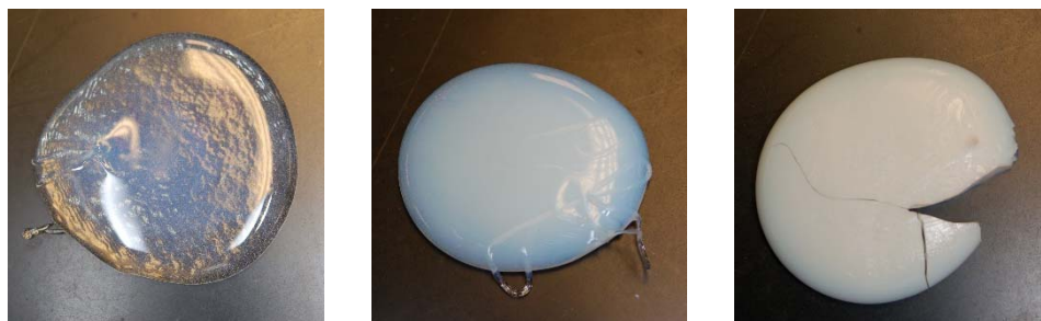
Figure 1-1. Examples of opalescent and opaque alkali borosilicate glasses that are phase separated.
