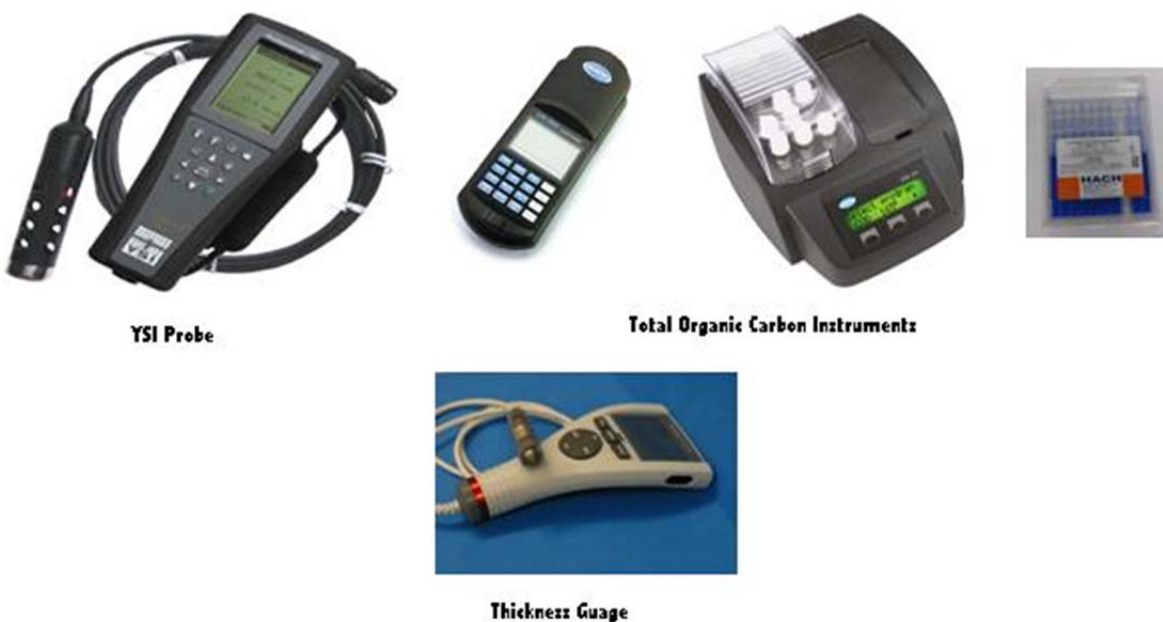
Figure 1. Spent Fuel Characterization Kit Components
