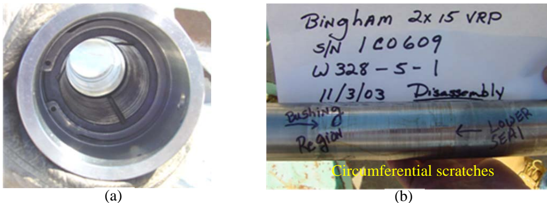
Figure 1. Bearing and shaft damage from contact on a disassembled SRS standard slurry mixing pump.
