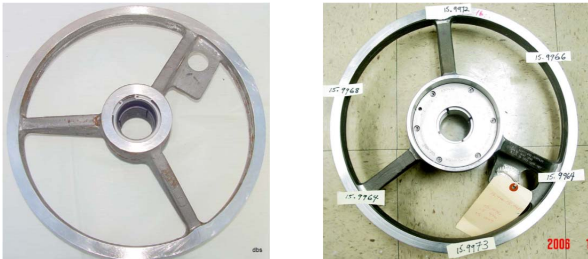
Figure 7. Unmodified QVSP spider bearing assembly which caused whirl vibration (a), and Modified QVSP spider bearing assembly which eliminated whirl vibration (b).
