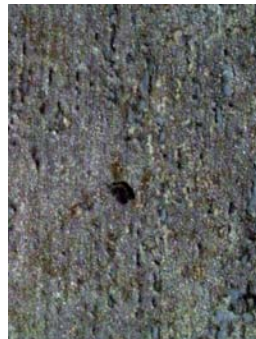
Figure 12. Cleaned Coupon showing pitting corrosion in (a) HM/2.5 wt.%oxalic acid at 75 °C with no agitation, (b) HM-PUREX/2.5 wt.% oxalic acid at 75 °C with agitation. Magnification was 20X unless shown otherwise.
