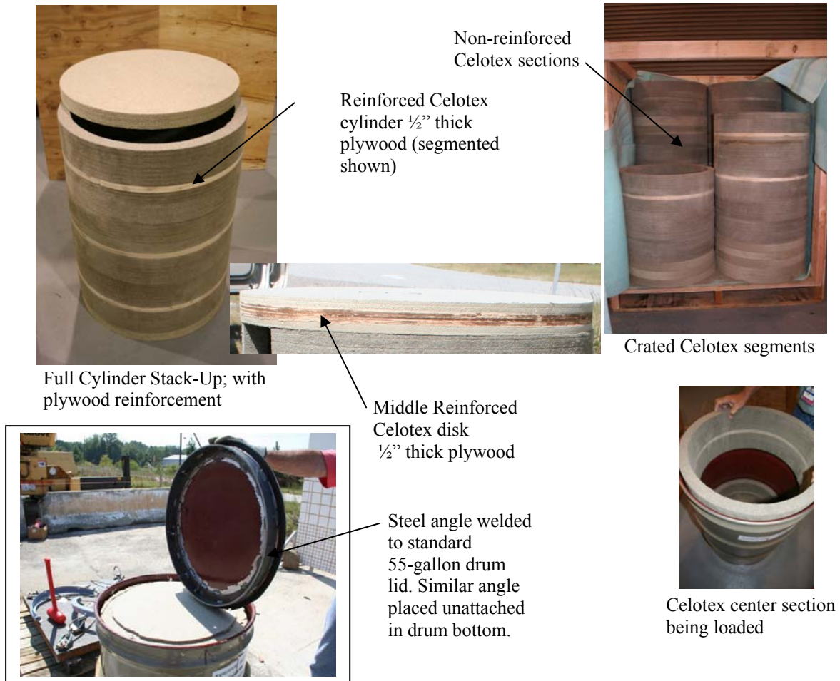
Figure 2 Celotex Assemblies and Reinforcements
