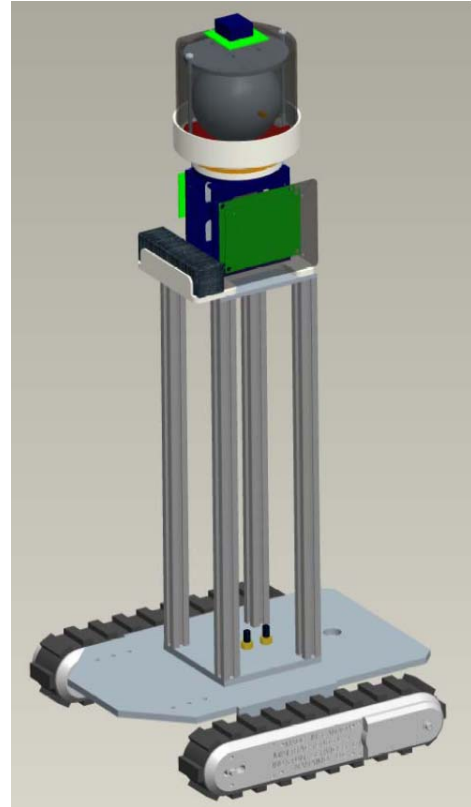
Fig. 3. RadBall Position and Orientation Device System on a robot (Images: SRNL)
