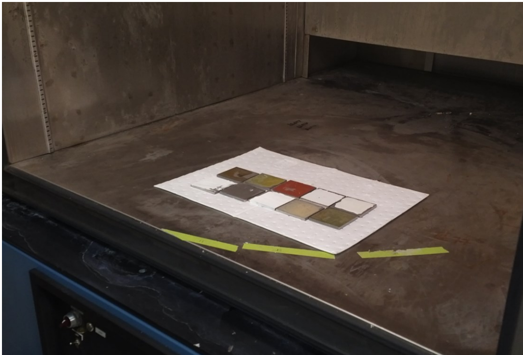
Figure 1: FCGs placed to cure in the environmental chamber.
