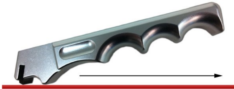
Figure 4: Cross-hatch Tool for Adhesion Testing
