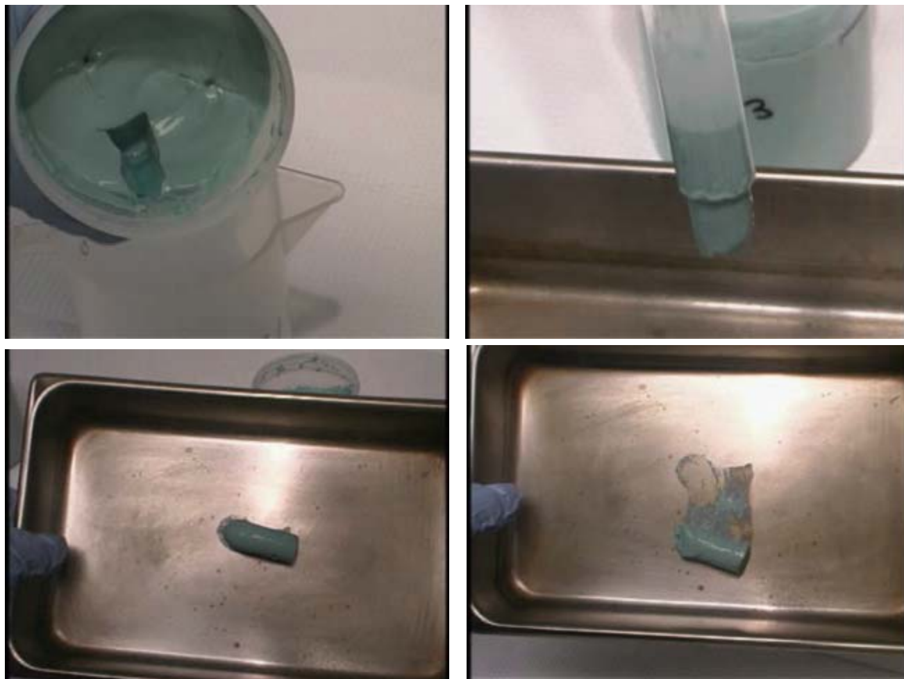
Figure 1. Kaolin Sample with 0.9 wt% magnesium aluminum silicate and 0.1 wt% sodium carboxymethylcellulose after 26 days
