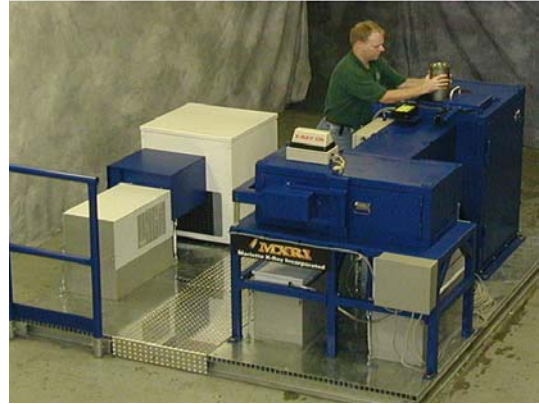
Figure 18: 420 kVp DR Cabinet Enclosure
