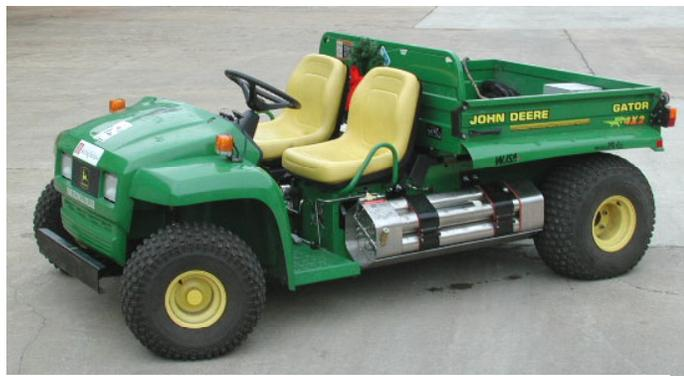
Figure 10. Picture of the Gator™ hydrogen fuel cell vehicle.
