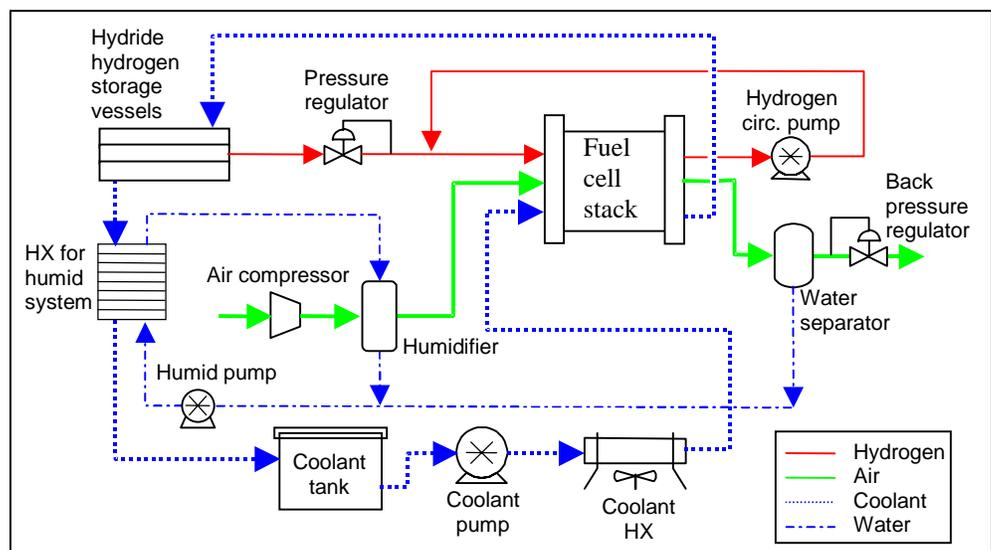
Figure 9. Hydrogen fuel cell power system for Gator<sup>TM</sup> utility vehicle.
