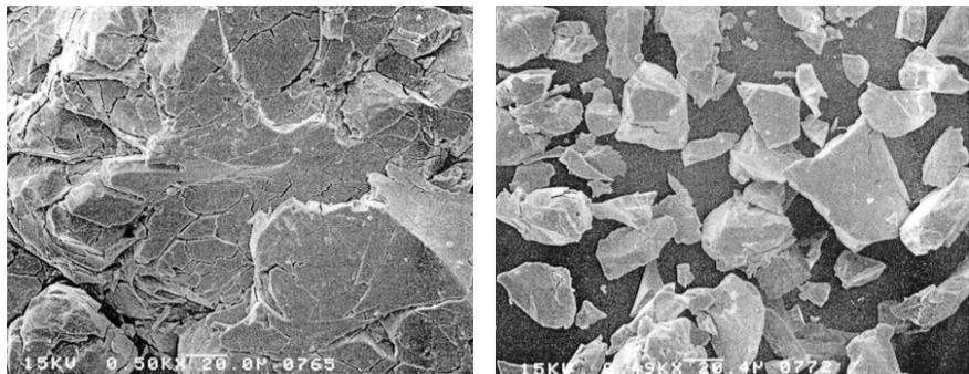
Figure 2. Metal hydride (LaNi<sub>4.25</sub>Al<sub>0.75</sub>) broke up to fine powder after repeated hydrogen absorption and desorption, 1 cycle (left) and 10 cycles (right).
