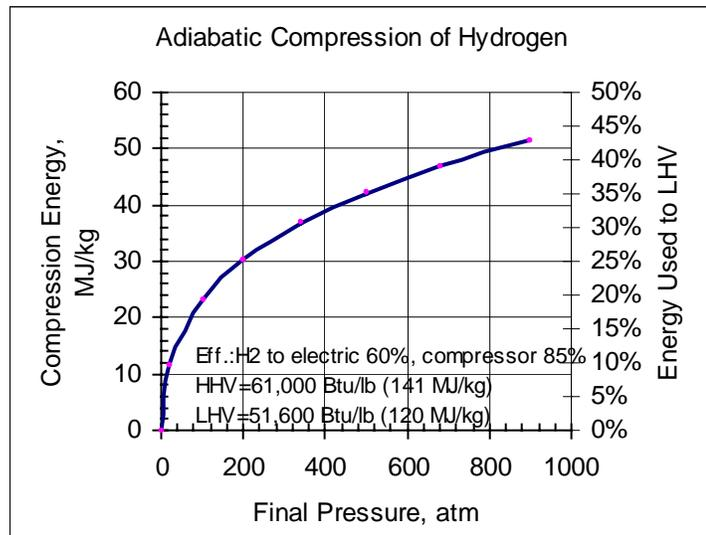
Figure 1. Energy consumption of compressing hydrogen.
