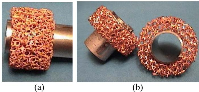
Fig. 6. Samples of 45 Sn 55 Cu brazed at 425°C. (a) Cu on external surface, 0.001" (b) Sn on external surface, 0.0005".
