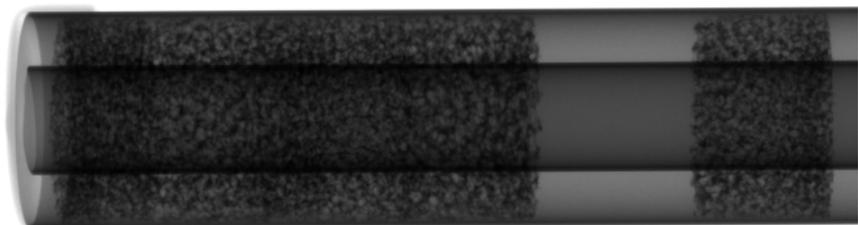
Fig. 11. X-ray radiograph showing the brazed assembly and tight packing of the foam disks on the left and a spaced disk on the right
