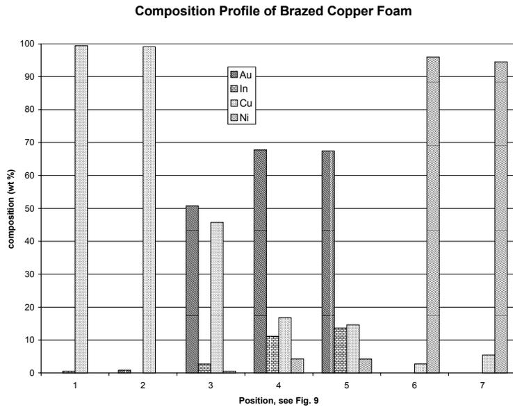
Fig. 10. Composition profile of brazed copper foam.
