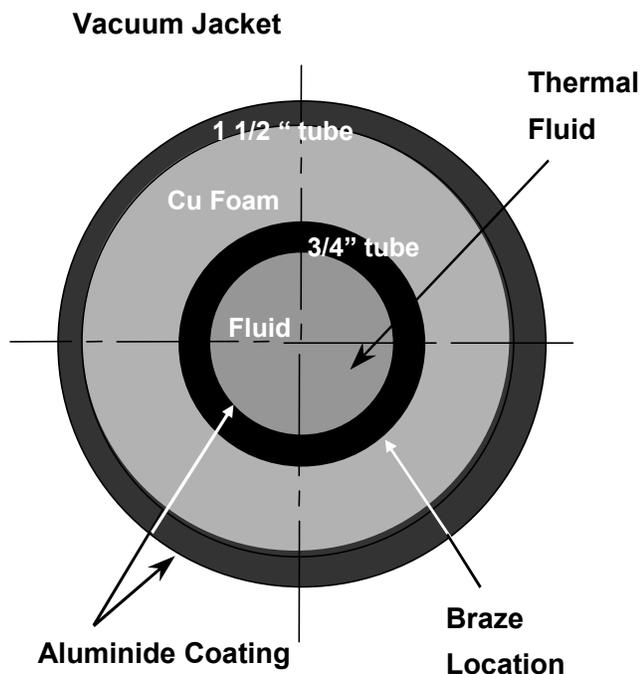
Fig. 2. Schematic cross-section of TnT TCAP.
