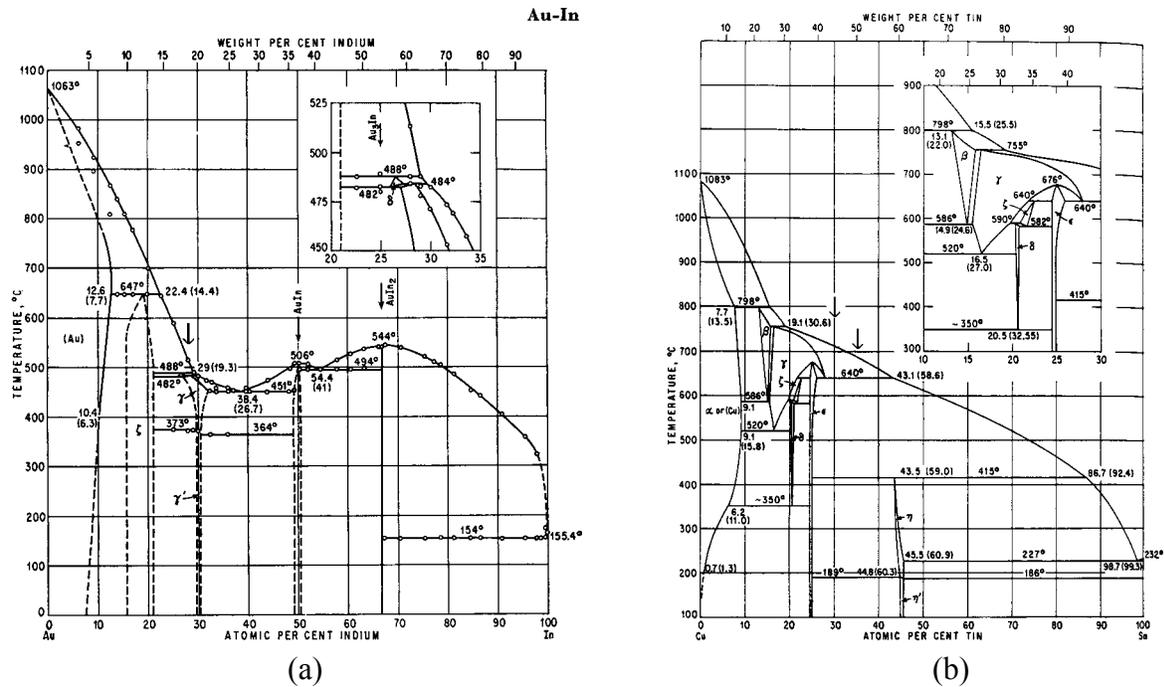
Fig. 4. (a) Gold-indium and (b) copper-tin phase diagrams. The alloys evaluated are indicated by the arrows.
