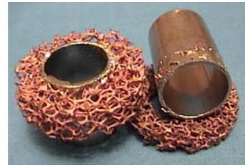
Fig. 7. Macrophotograph of foam brazed using Au/In and bond strength tested.
