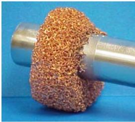
Fig. 5. Copper foam piece brazed to type 316L SS using Au-Cu at 980°C.
