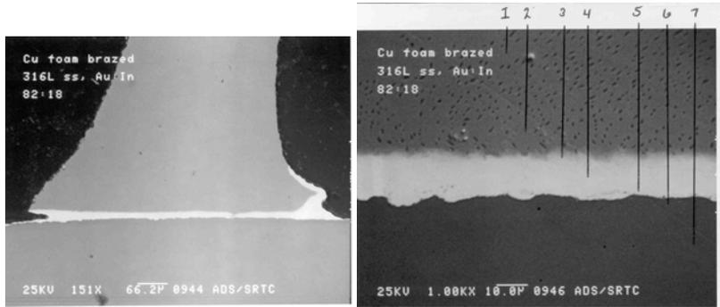
Fig. 9. SEM micrographs of brazed copper foam.
