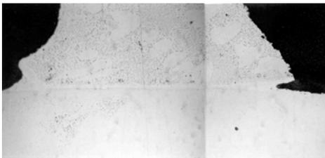
Fig. 8. Optical micrograph of Au-In brazed corner foam (200X).
