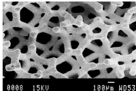
Fig. 3. Low (0.83X) and high magnification images of the copper foam used for the brazing study. Actual pieces had holes drilled in the center to accommodate the inner tube.
