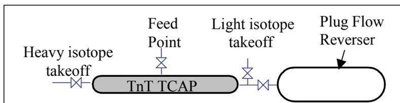
Fig. 1. Typical TCAP design layout.
