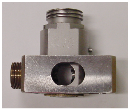
Fig. 1. Weld fixture for confined pinch welds.
