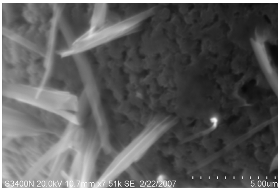
Figure 7. Nano-Structure Absorbent Grown Outside PW-HGMs
