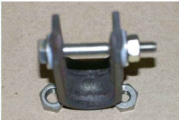
(c) Compressive side of U-bend before exposure
