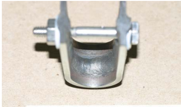
16747 (c) Compressive side of U-bend before exposure
