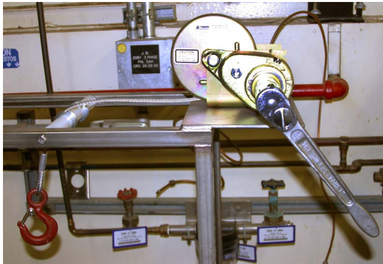
Figure 22 Winch assembly for lifting and lowering the plate specimens.
