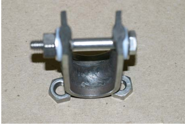
(c) Compressive side of U-bend before exposure
