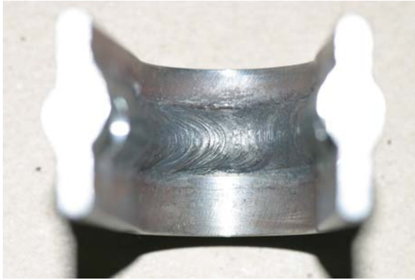
(c) Compressive side of U-bend before exposure
