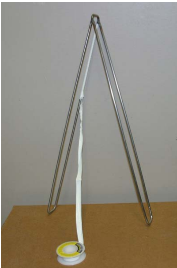
Figure 21 Insulating of rack with Teflon tapes.
