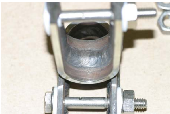
(c) Compressive side of U-bend before exposure
