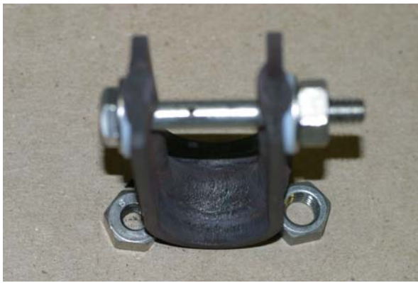
(c) Compressive side of U-bend before exposure
