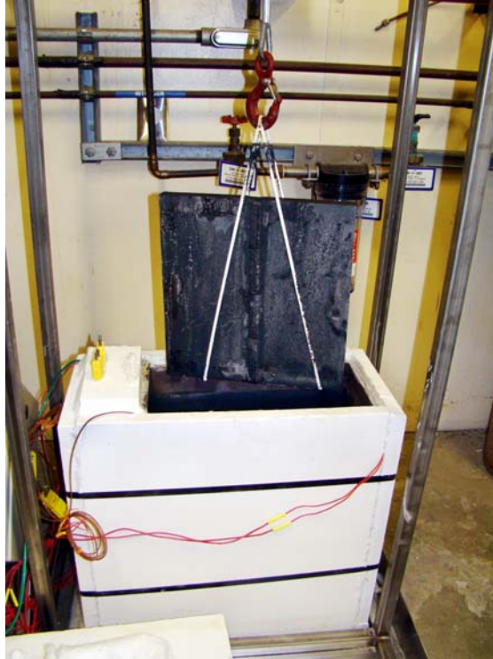
Figure 24 Periodic inspection for cracking by lifting plate above the test solution.
