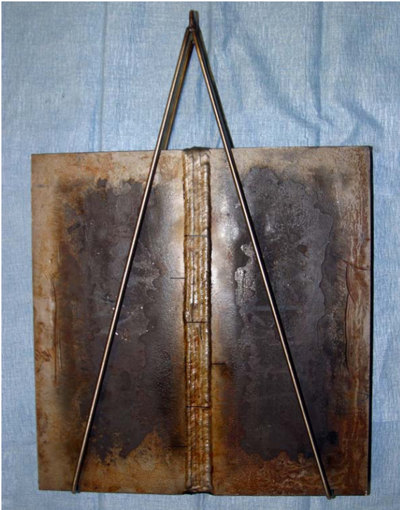
Figure 19 Positioning of the test plate on the rack (hanger).
