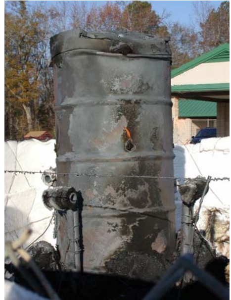
Figure 2. Typical 9977 package following fire test.
