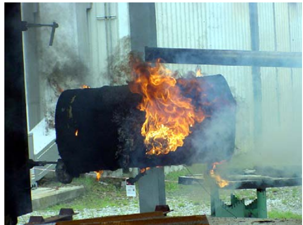
Figure 4. Package removed from furnace at end of thermal test. Flames are burning gaseous decomposition products.
