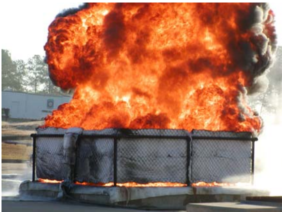
Figure 1. Pool fire test of 9977 package.
