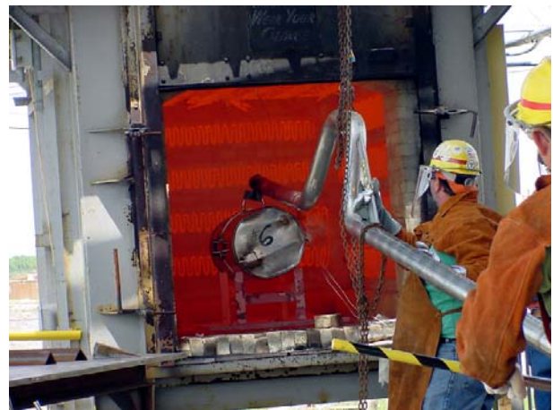
Figure 3. Furnace test of GPFM prototype.
