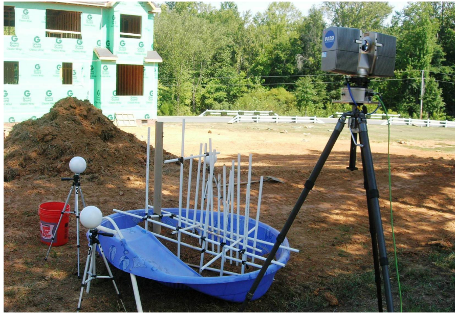
Figure 15. Volume determination of the solids placed in the test mockup
