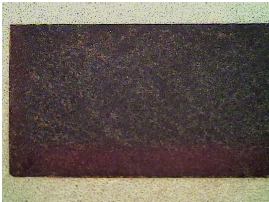
Figure 4-16. Electrode micrograph after exposure to magnetite in 0.1 M nitric and 1 wt. % oxalic acids at 75 °C (magnification 1x).
