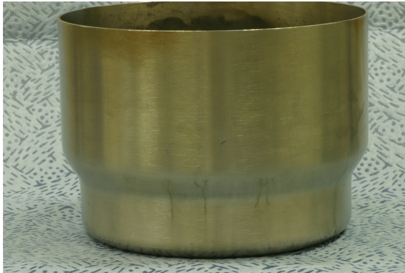
Figure 11. Convenience container section after exposure to boiling magnesium chloride solution: container exterior with axial cracks in sidewall
