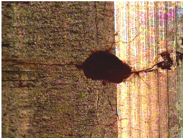
Figure 9. 3013 inner-container welded-top section after exposure to boiling magnesium chloride solution showing pit associated with cracking in sidewall
