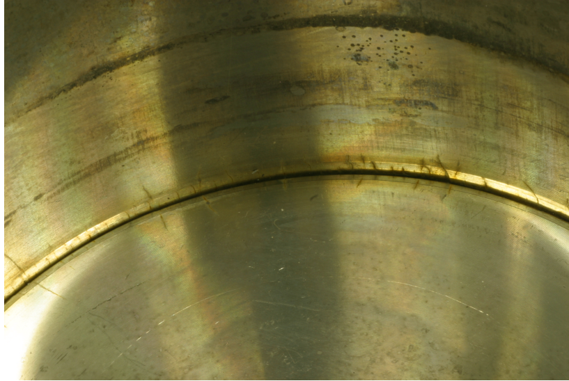
Figure 8. 3013 inner-container welded-top section after exposure to boiling magnesium chloride showing container interior with sidewall and plug cracks
