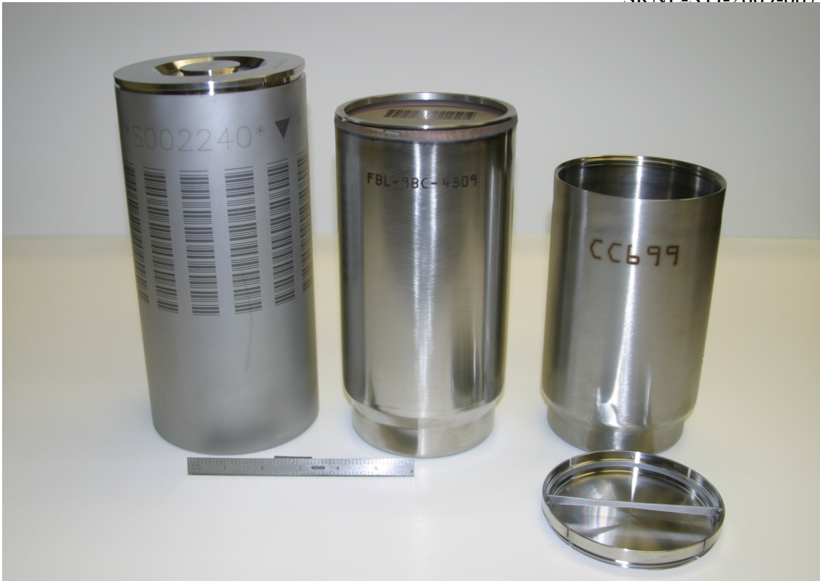
Figure 1. 3013 containers (outer, inner, convenience) used by Savannah River Site for oxides
