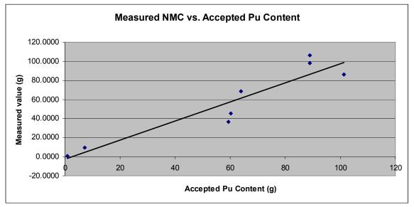
Verification Measurements with eight standards used for qualification of the portable active well coincidence counter for passive neutron multiplicity measurements of Pu in the range 0.78 – 101 g.
