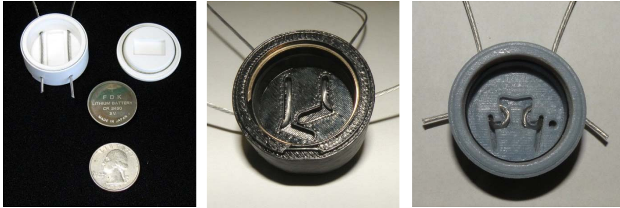
Figure 3: Left, Gen I Wire Routing. Center & Right, Gen II Wire Routing Options. Photos courtesy of SNL & SRNL.
