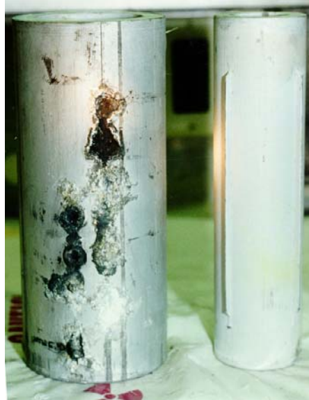
Figure 2 Mk-31 Outer and Inner Target Tubes. The tubes are aluminum-clad uranium metal.
