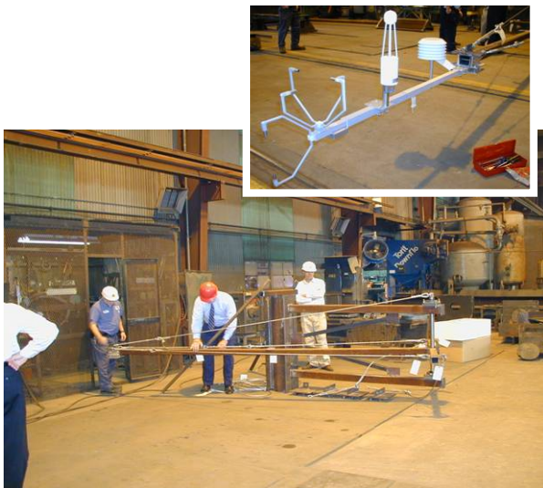
Fig.11 Instrument boom flexed in the middle to demonstrate instrument change-out for calibrations. These booms were designed and constructed by Kline Towers Inc., the company that designed and built the WJBF-WAGT-TV tower.
