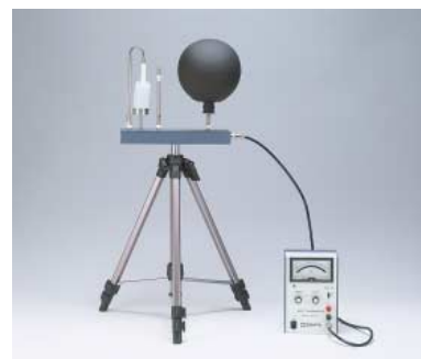
Fig. 15 Labor intensive Wet Bulb Globe Thermometer.
