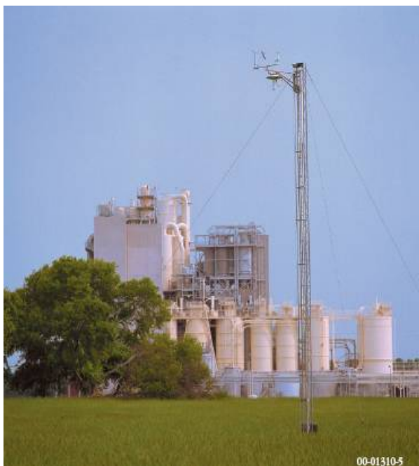
Fig. 8 The meteorological tower at the Proctor & Gamble Augusta plant. Data is transmitted every 15 minutes to the SRS meteorological Weather Information and Display (WIND) System. Data is available to the surrounding county and state emergency managers.
