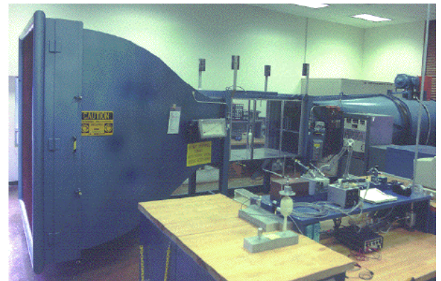
Fig. 12 SRNL Wind tunnel for instrument testing and calibration.
