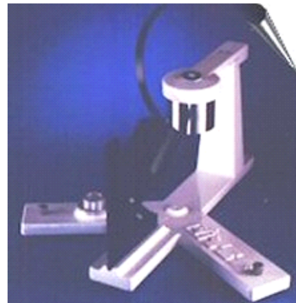
Fig. 7 A Multi-Filter Shadow Band Radiometer to measure direct and diffuse solar radiation – an example of instrumentation at the Climatology facility.
