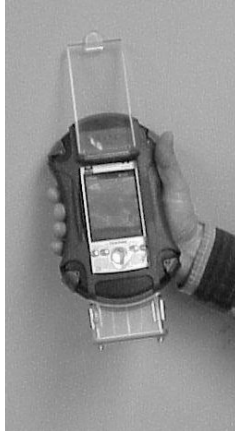
Fig. 8. PDA In Ruggedized Housing
