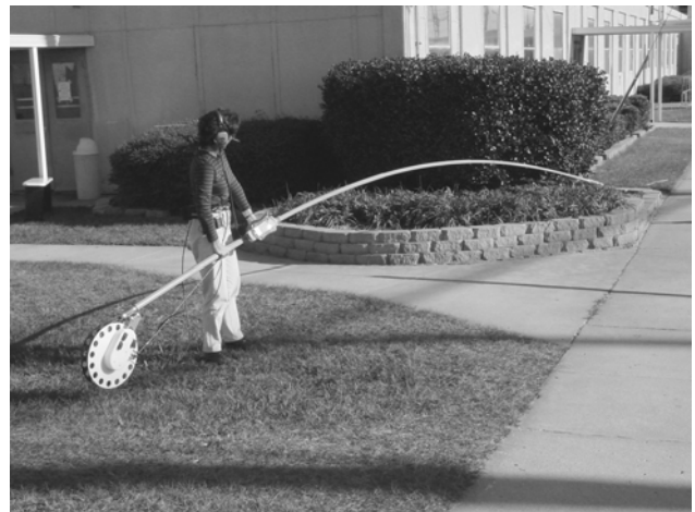
Fig. 2. RPC Deployed In Horizontal Extension Form
